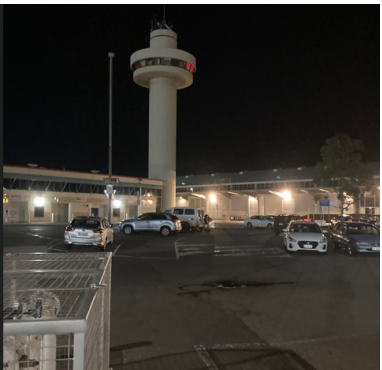
West of port building: Lighting levels ranged from 1 to 30 lux. Lighting is provided by building mounted lights - from the port building and the red brick building the west side of the car park (LED)
