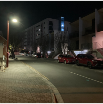
Creswells Row: Lighting levels ranged from 1 to 20 lux. Lighting is provided by pole mounted luminaires, which appeared to be metal halide or high pressure sodium lamps.
