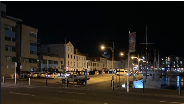
Hunter St: Lighting levels ranged from 3 to 40 lux. Lighting is provided by pole mounted luminaires, which appeared to be metal halide or high pressure sodium lamps.
