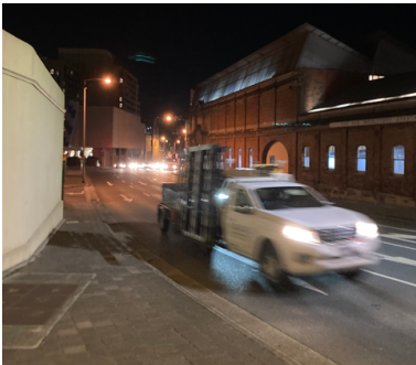
Macquarie St: Lighting levels ranged from 5 to 40 lux. Lighting is provided by pole mounted luminaires, which appeared to be metal halide or high pressure sodium lamps.
