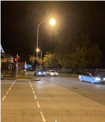
Davey St: Lighting levels ranged from 6 to 40 lux. Lighting is provided by pole mounted luminaires, which appeared to be metal halide or high pressure sodium lamps.
