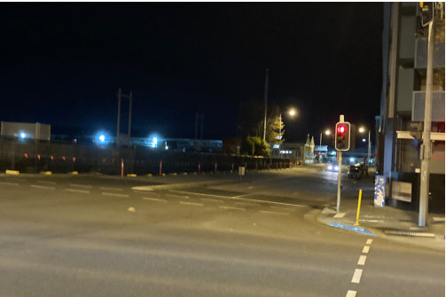
Evans St: Lighting levels ranged from 1 to 40 lux. Lighting is provided by pole mounted luminaires, which appeared to be metal halide or high pressure sodium lamps.
