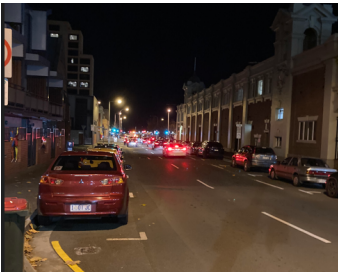
Campbell St: Lighting levels ranged from 1 to 20 lux. Lighting is provided by pole mounted luminaires, which appeared to be metal halide or high pressure sodium lamps.
