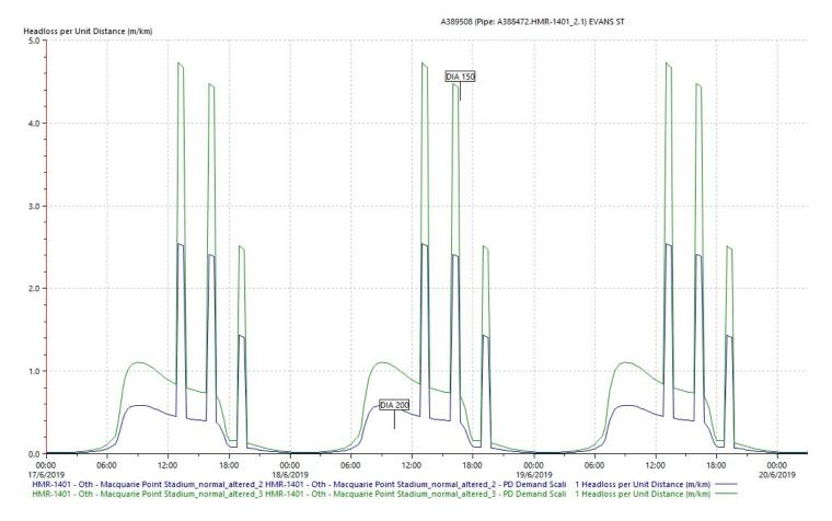
A final chart shows headloss in the high way crossing, which does not drop below 5.0m/Km in any of the simulations. We have assumed that augmentation across the highway is not ideal, as this would need to extend back to Campbell Street either along Brooker Avenue and the Collins Street or along Macquarie Street, both of which have significant services to cross including the Hobart Rivulet, Selfs Point to Blinking Billy Pipelines and the Mac Point Trunk Sewer
