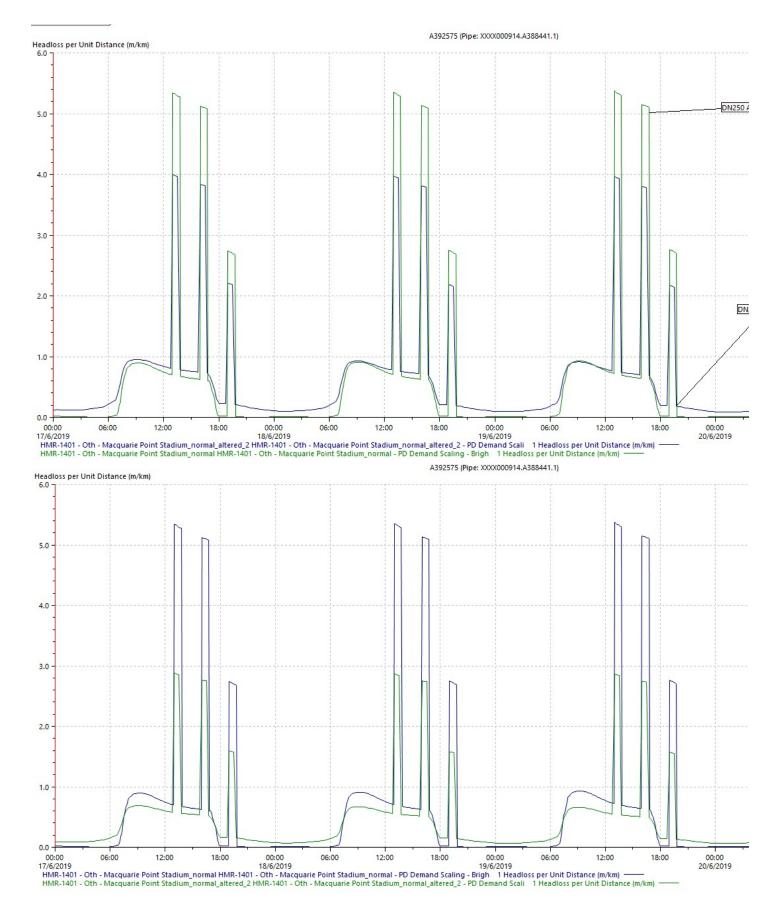
For Evans Street headloss is very high in the existing main to Connection point 2, with a 150mm augmentation headloss reduces to just under 5.0m/km.
