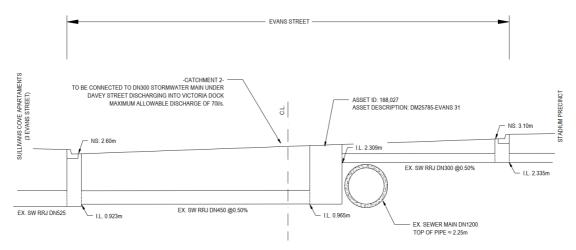
Figure 5 - Catchment 3 Evans Street Stormwater
