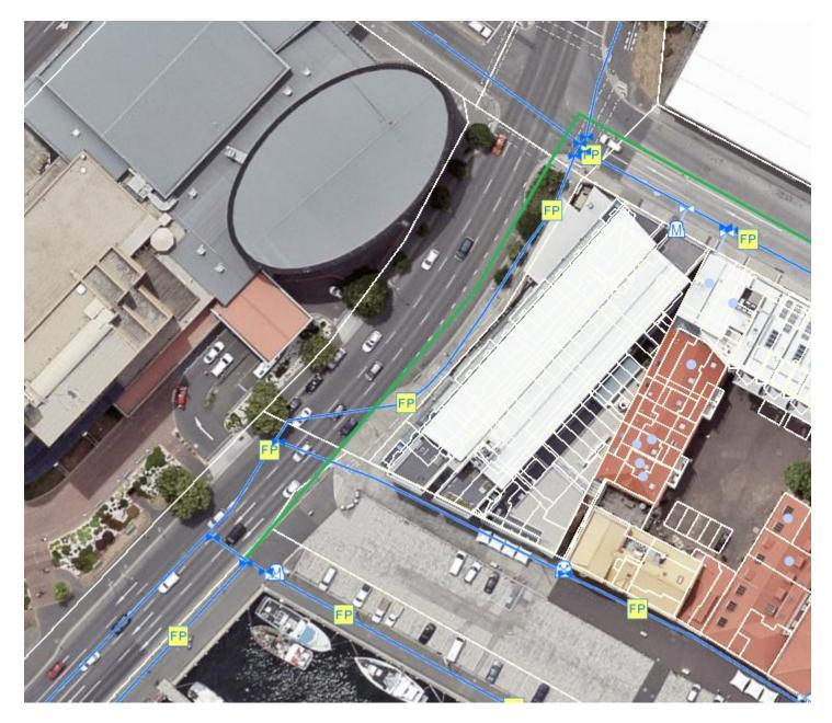
It should also be noted that MPDC previously constructed a water main along the road from connection point 1. This pipe likely requires replacement to facilitate the stadium, if it is replaced, and the pipe is to ultimately be gifted to TasWater, it should be sized such that headloss in the pipe is below TasWater standards for the design flows. Once beyond the connection to the stadium in this scenario the pipe may be reduced to a smaller size if modelling confirms it is appropriate.
